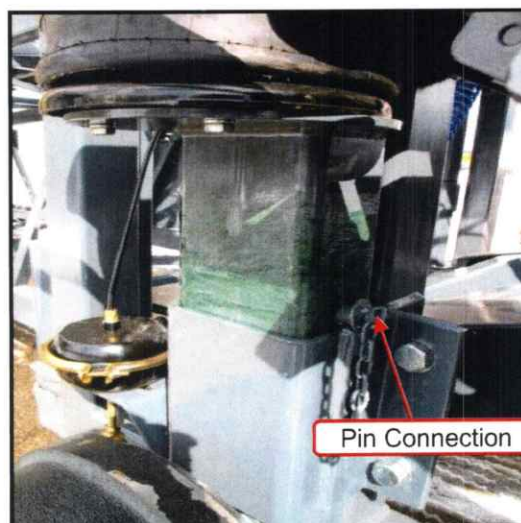
Picture 3-16: Auxiliary Axle Airbag
