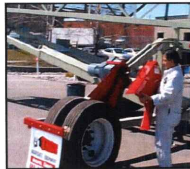
Picture 3-23: Installing Drive Chain
