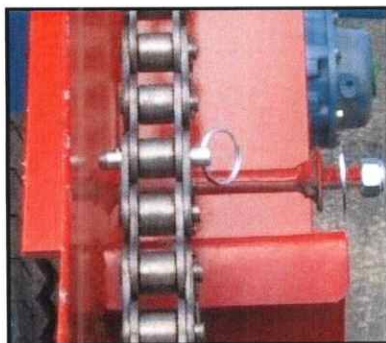
Picture 3-22: Installing Drive Chain
