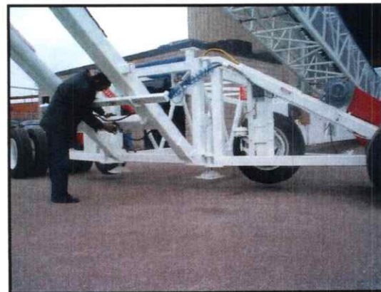
Picture 3-11: Adjusting the Hydraulic Flow Control
