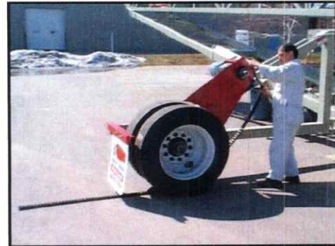
Picture 3-20: Installing Drive Chain
