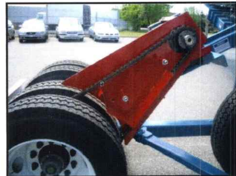
Picture 3-21: Installing Drive Chain
