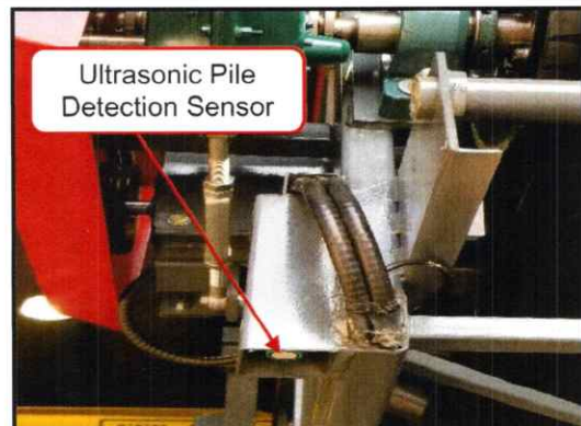
Picture 3-4: Ultrasonic Pile Detection Sensor
